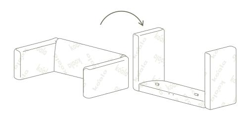
Screw baseboard with green lining up, onto frame using long thread legs in the order shown.
